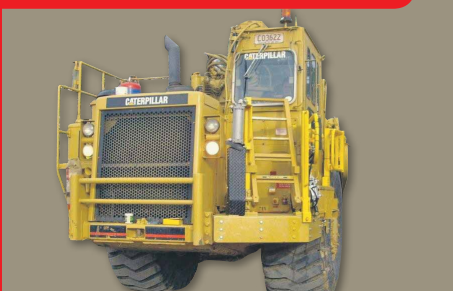
ACCESS SYSTEM IN OPERATION MODE - FOLDS WITHIN SCRAPER'S FOOTPRINT
